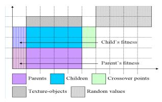
Figure 7: Framebuffer data structure, shown as a grid of single pixels. Individuals' chromosome strings are ordered in horizontal manner. Texture data for one texture and genes are stored within one pixel.
