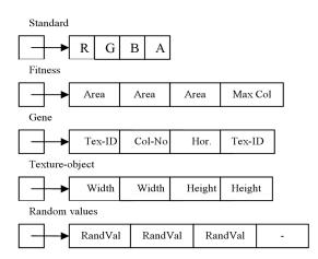
Figure 8: Different pixel data formats using RGBA texture format. "Tex-ID" is a reference to a texture. "RandVal" stores a random value (between 0-255). "Col-No" refers to a column number. "Hor" is set when textures should be rotated. "Max. Col" refers to the number of columns a solution possesses.
