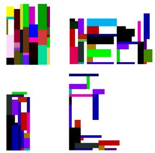
Figure 16: Results of the space optimization: lower pictures show the left-shifted approach. On the lower right, a bad solution for 20 textures can be seen. On the lower left, a good solution for 20 textures. On the upper right, a bad solution for 30 textures. On the upper left, a good solution for 30 textures. Good solutions are calculated after few generations.
