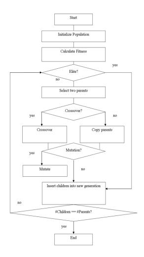
Figure 1: Typical work flow chart for processing one generation of a genetic algorithm.
