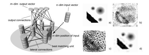
Fig. 1. On the left side, an example SGCS network is outlined. The output connections are drawn for four input cells only. On the right side, a two-dimensional example goal function (a) is approximated (d). (b) and (c) show the samples which are selected by the algorithm and the created network structure.
