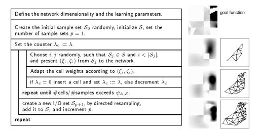
Fig. 2. The extended basic algorithm for the SGCS network, and a running example which shows growing and the adaptive function approximation of the goal function.
