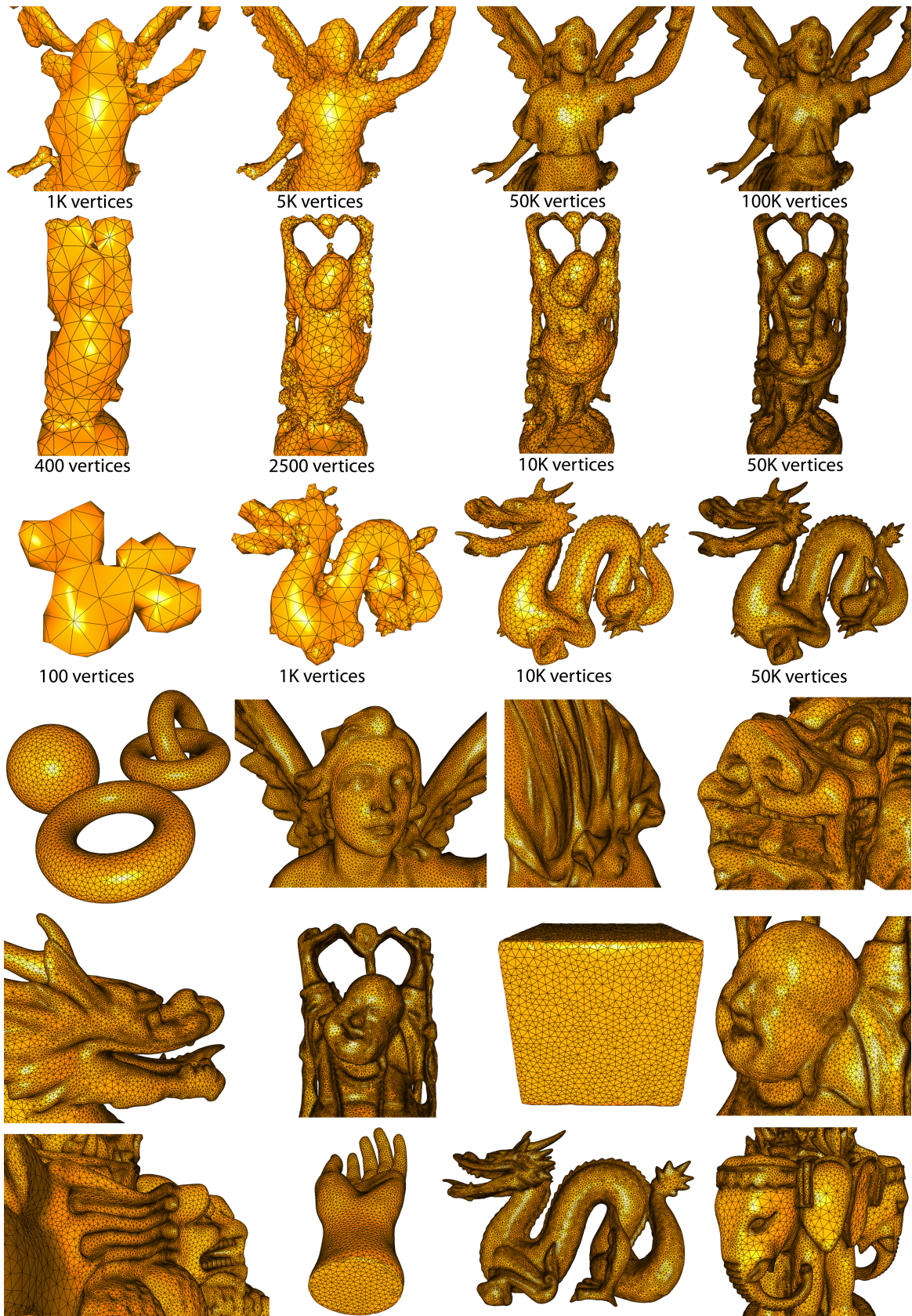
Figure 16: Upper lines: mesh training stages with number of vertices, lower lines, assorted pictures of reconstructed models.
