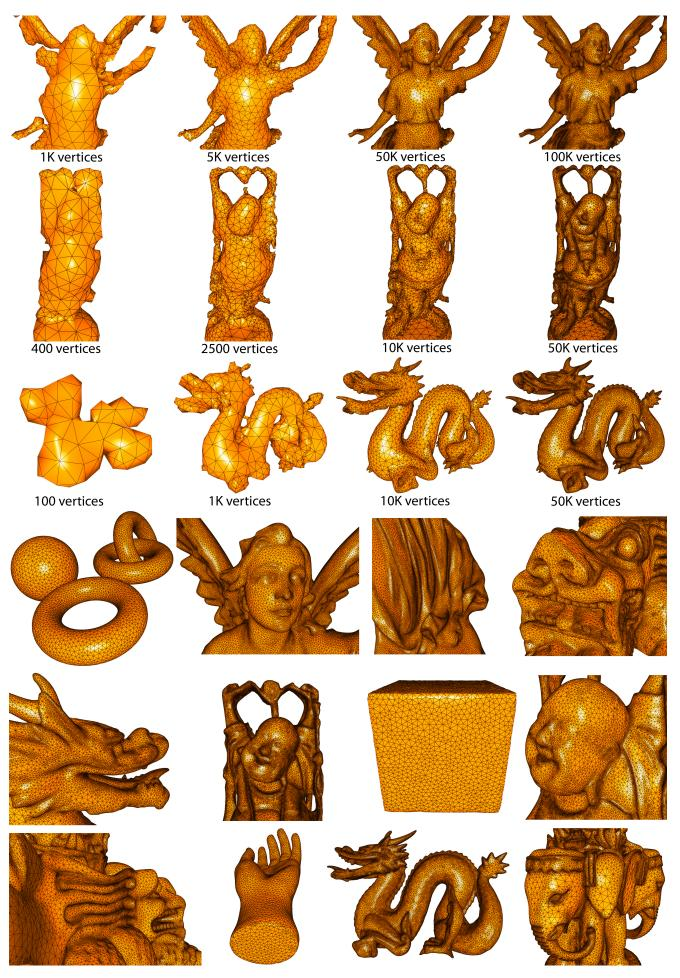
Figure 14: Upper lines: mesh training stages with number of vertices, lower lines, some assorted pictures of reconstructed models.
